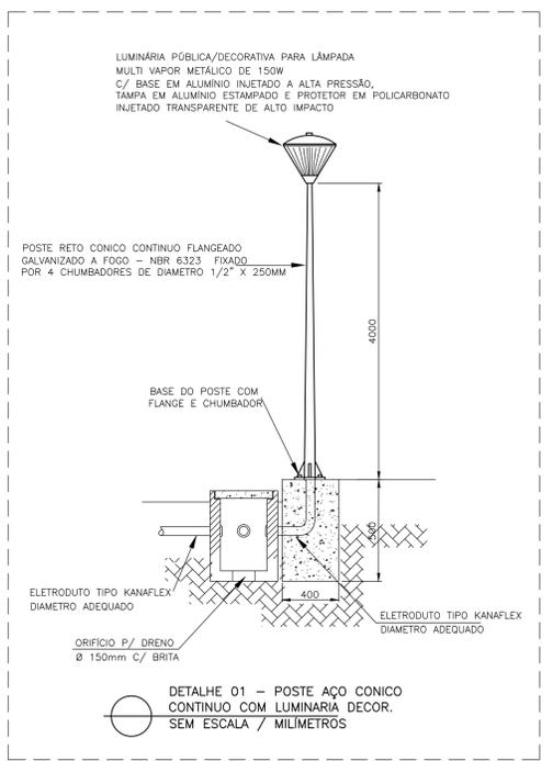
DETALHE 01 - POSTE AÇO CONICO CONTINUO COM LUMINÁRIA DECOR. SEM ESCALA / MILÍMETROS
