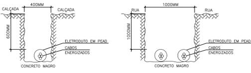
DETALHE - 18: VALA PARA CABOS E ELETRODUTOS SEM ESCALA
